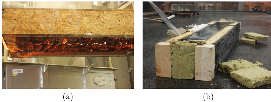
Figure 5.4: Fire test termination: a) removing samples, b) extinguishing samples.
