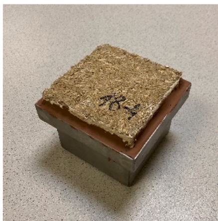
Fig. 3. Determination of water vapor permeability (left) and an example of the manufactured sample (right).
