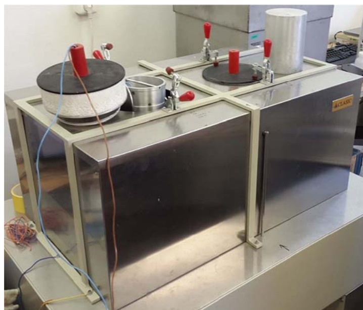
Figure 3.1. Isothermal heat flow calorimeter.
