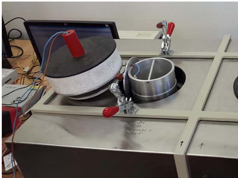
Figure 3.2. The aluminum calibration insert.
