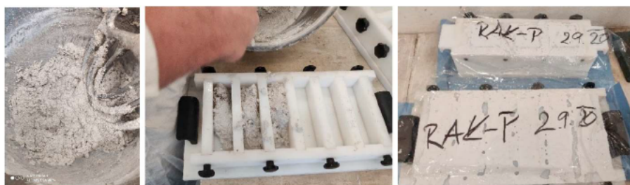
Fig. 2 – Production process of cement composites.
