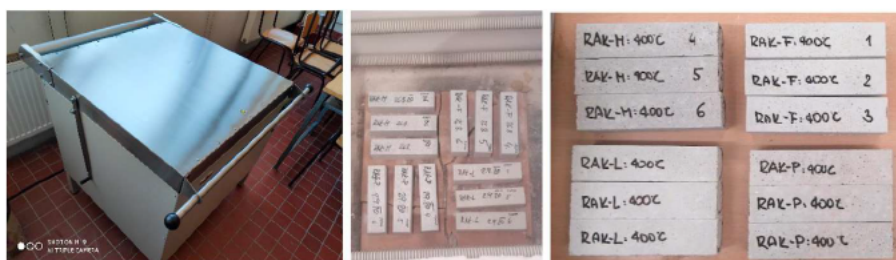
Fig. 3 – Thermal loading of cement composites.
