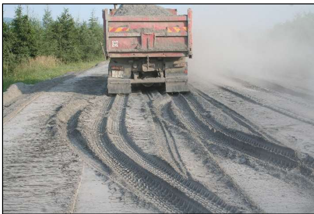
Figure 2. Bulk density of the ash was determined in the field using a Tatra 815 truck.
