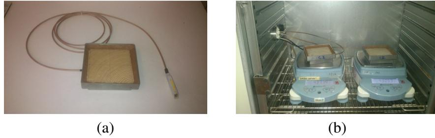
Figure 2: Cup method: a) measured sample, b) testing chamber
