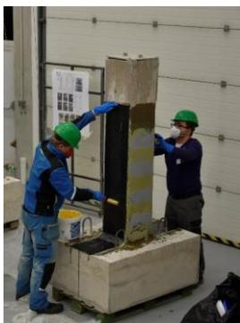
Step 13-CFRP sheet wrapping
