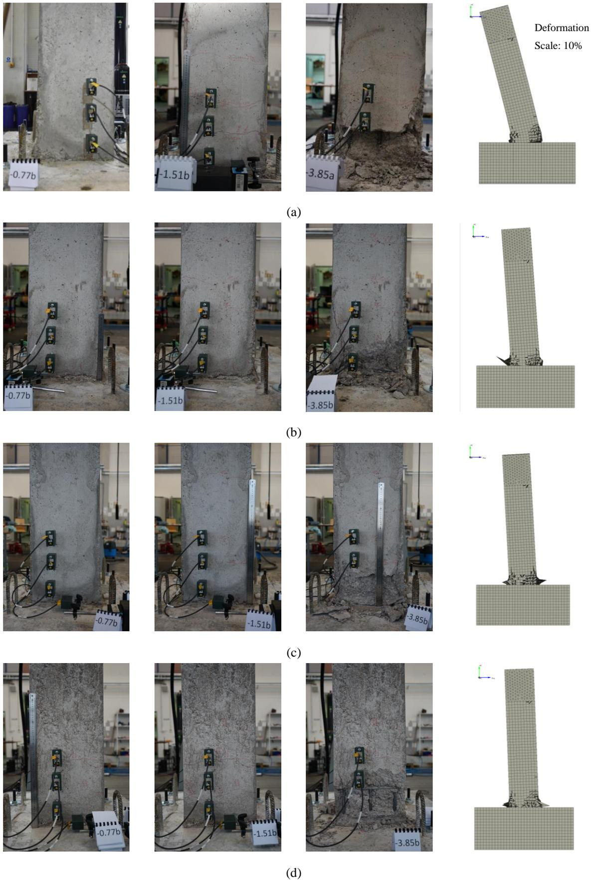
Fig. 4.2. Damage evaluation in as-built specimens (a) E1-T-H (b) E1-C-H (c) E1-NC-H (d) E1-T-L (e) E1-C-L (f) E1-NC-L.
