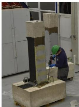
Step 14-Chemical anchor for fiber anchors
