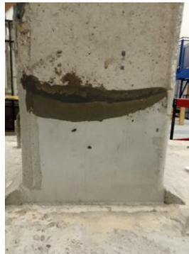
Step 7-Crack filling by epoxy injection
