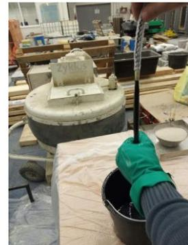
Step 8- Wet epoxy resin application for fiber anchor
