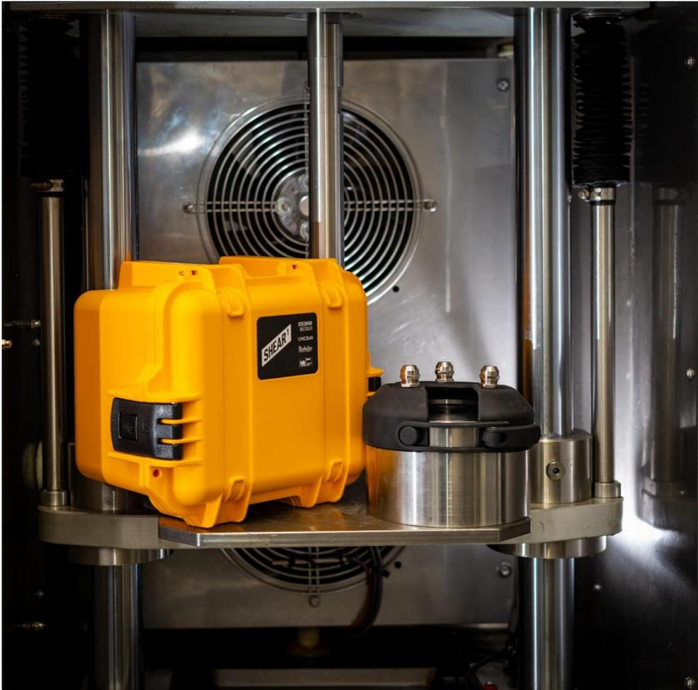
Figure 3. The Uniaxial Shear Tester (2<sup>nd</sup> prototype) placed in the temperature chamber at Department of Road Structures, Czech Technical University in Prague, 2020
