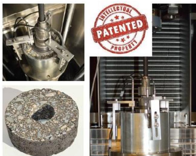
Figure 4. Universal Shear Tester
