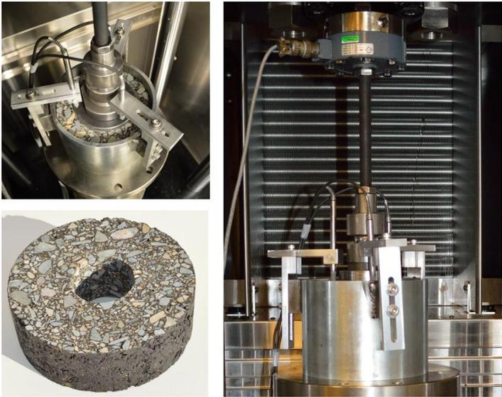
Figure 2. Uniaxial Shear Tester (top view, hollow cylindrical specimen, UST placed in UTM chamber)
