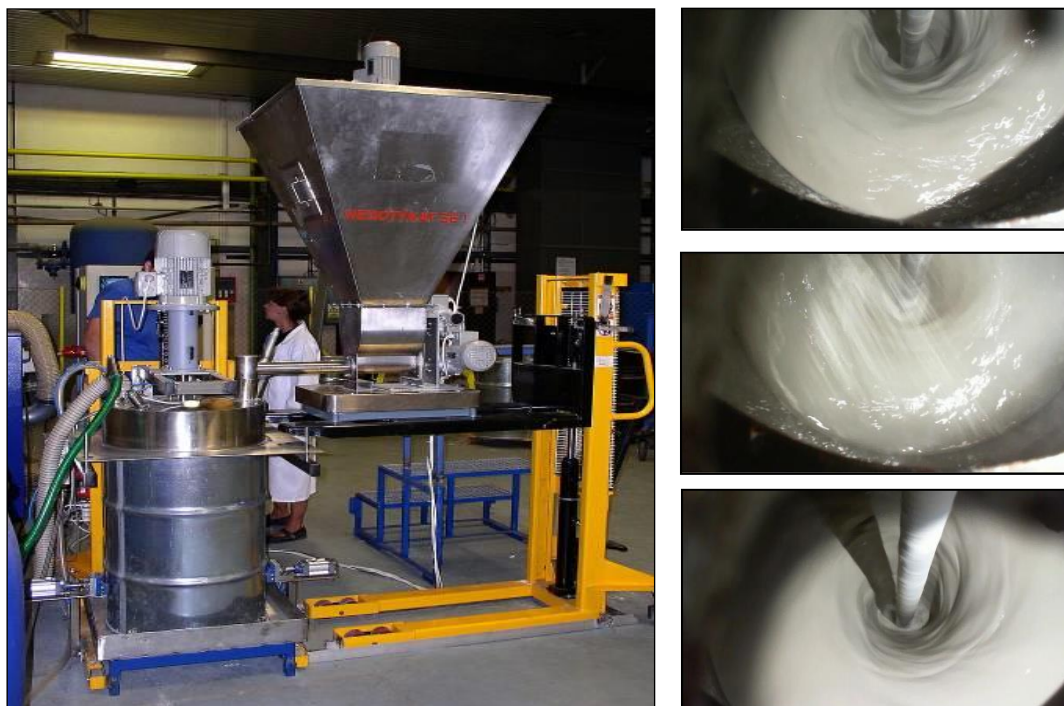
Figure 1-3: Testing of solidification of semi-liquid radioactive waste in UJV Řež in cooperation with Chemcomex Praha a. s., Czech Republic (Trtílek, 2017)
