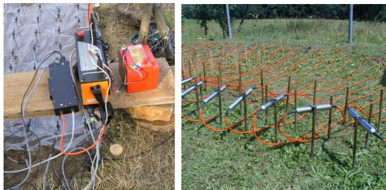
Figure 11. Electric resistivity tomography monitoring system (ARES, GF Instruments, Brno)
