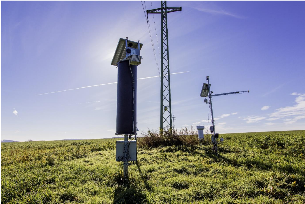
Figure 10. Cosmic rays neutron sensor (Styx Neutronica, Germany) and the meteorological station on the Nučice catchment (photograph by T. Li)
